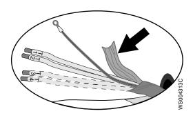
Figure 10: Copper foil on control element.
