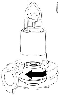
The correct direction of impeller rotation is clockwise when you look at the pump from
