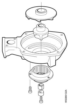
Figure 18: M-impeller
