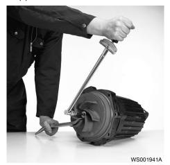
Check that the impeller can rotate freely.
