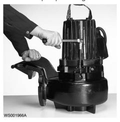
2. Remove the impeller screw. If applicable, use the rod.
