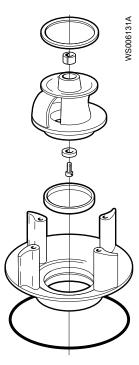
Figure 15: L-impeller
