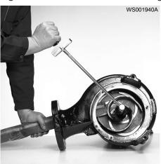
Check that the impeller can rotate freely.
