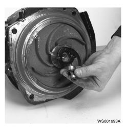
4. Fit the impeller puller and pull off the impeller and cutting wheel. Place a protector between the screw head and the impeller puller.
