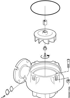
Figure 14: D-impeller
