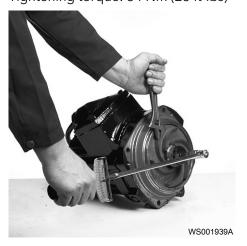
Check that the impeller can rotate freely.
