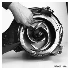
b) Tighten the impeller screw.
