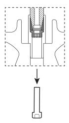
b) Remove the impeller.
