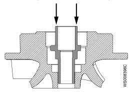
2. Check that the adjusting screw is correctly positioned in the new impeller.
