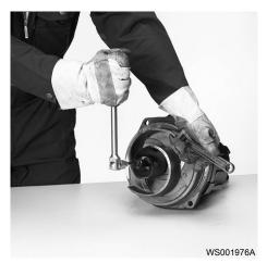
Remove the impeller.
