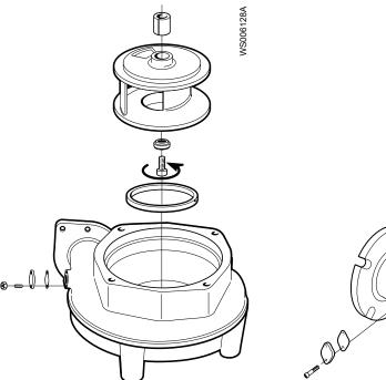
Figure 13: C-Impeller
