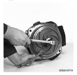
3. Refit the impeller screw.
