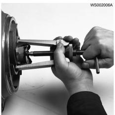
5. Remove the conical sleeve.
